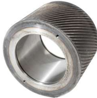
Corrugated Helical (HTWH, 13c, 14o) Designed with corn-based animal feed in mind. They work well in a three-roll set up and tend to do a better job cleaning off the die pad.
